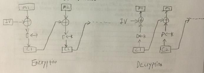
Note: The IV is sent encrypted in the first packet by the sender.
